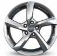
19" x 8.5" Front and 20" x 10" Rear Aluminum Torque Directional Wheel in Chrome
