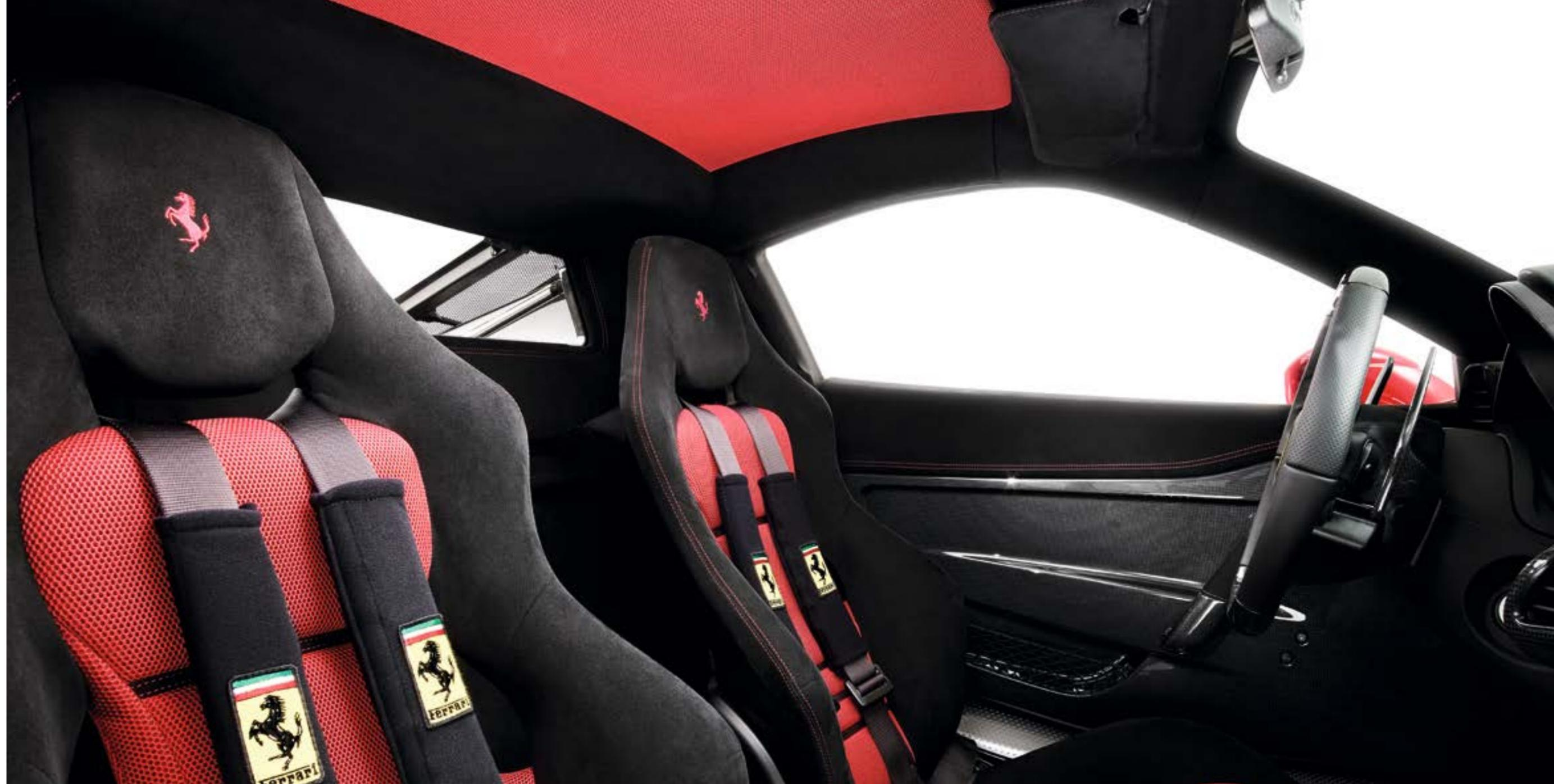
The Sabelt seats have carbon-fibre shells and boast excellent side bolstering thanks to an ergonomic design which also helps contain weight. The shoulder-rests are trimmed in Alcantara for improved grip while seated and the backrests are padded with a breathable 3D fabric to guarantee excellent air circulation and comfort. The same anthracite Alcantara trim with contrasting red stitching also adorns the dash, the door panels, interior and posts.
