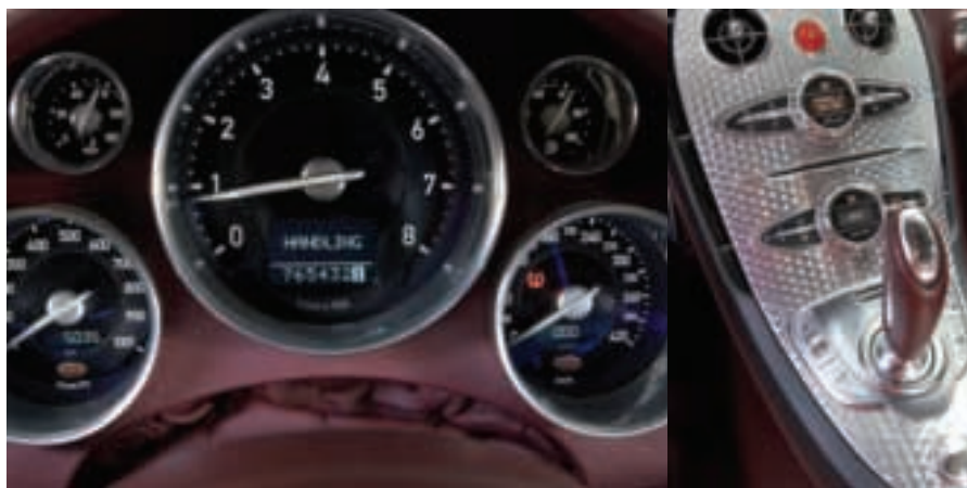
Veyron speedometer reads up to 420 km/h; left-hand gauge shows horsepower deployed
