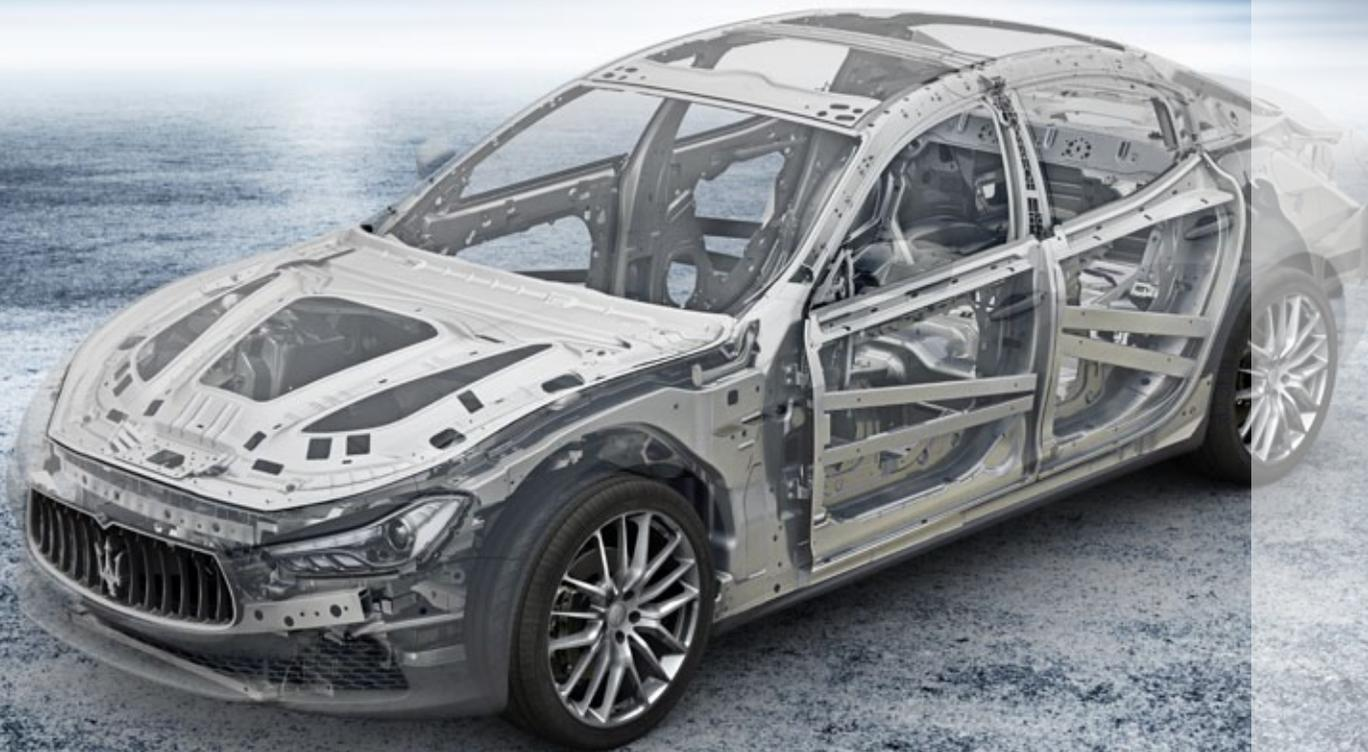
The Maserati Ghibli's stunning design has been made possible thanks to a brand new frame that is constructed from aluminium alloy to achieve strict weight and strength targets. For a car with a three metre wheelbase (the longest in its class) the Ghibli's roadholding and handling are outstanding, whilst its occupants enjoy the highest levels of safety.
